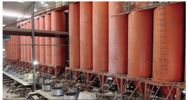
A batch storage system which can reserve 12,000 tons of prepared clay material
